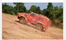
• 4 ×4 full-wheel driving, double-speed full-time transfer case, with differential lock, modular large-stroke double-fork highperformance independent oil-gas suspension system, with average crossing vehicle speed reaching 50km/h, with maximum climbing gradient of 60%.
