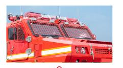
Anti-smash: Anti-smash: The frame-type independent cab can resist the vertical load impact of 100kg steel ball which falls from 20m height.
