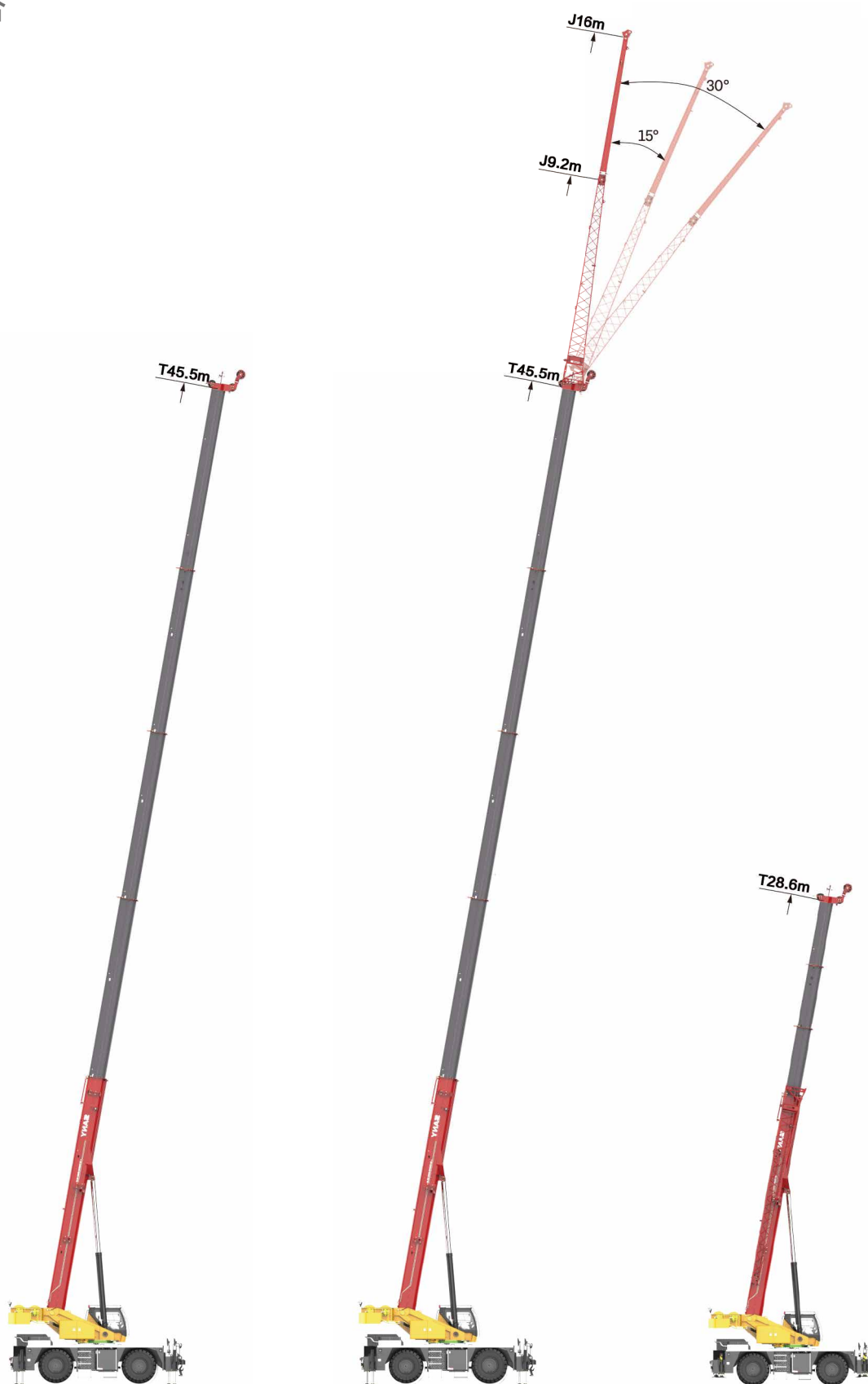
Telescopic boom on outriggers 主臂、支腿吊载
